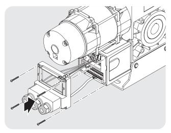
Place the limit switch cover onto the limit switch box.Tighten the screws on the limit switch cover plate.
