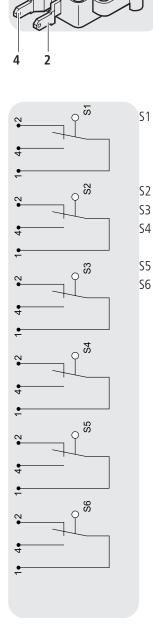
OPEN additional limit switch (standard only in the case of drives without integrated control unit) Limit switch, OPEN Safety limit switch, OPEN Safety limit switch, CLOSED Limit switch, CLOSED Additional limit switch, CLOSED (standard only for drives without integrated control unit)
