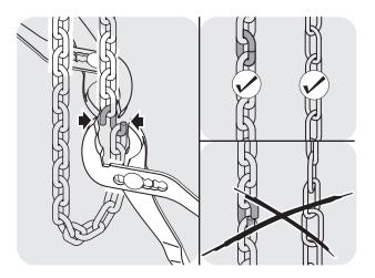
So in the ends of the emergency hand chain together with the chain connecting link.
