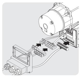
$\mathbb{I}$  Insert the cable set plug into the limit switch circuit board.
