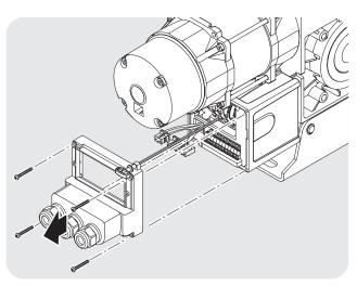
Remove the screws from the limit switch cover.Lift the limit switch cover off the limit switch box.
