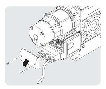
Place the adjustment cover onto the limit switch cover.Tighten the screws on the adjustment cover.
