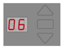
Simultaneously press and hold the 'UP' and 'DOWN' until the LED display shows '06', then press the "SET" button. Press the 'UP' or 'DOWN' buttons to increase or decrease the partial opening height. Number 1 indicates 10cm, number 2 indicates 20cm, the number 3 indicates 30cm. The number 20 indicates 200cm and so on. Press the 'SET' button to confirm your preferred settings.
