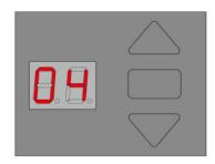
Press and hold the "SET" button until the LED shows the figure "O4". Press the "UP"button to increase the auto close time. Press the "DOWN" button to decrease the auto close time. Press the "SET" button to confirm the settings. When the auto close function is activated, the fully opened door will automatically close after the set time. The auto close function will be disabled when the LED shows O.
