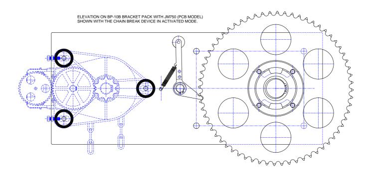
THIS IS A CHAIN BREAK DEVICE IT DOES NOT PROTECT AGAINST SINGLE COMPONENT FAILURE A SEPARATE ANTI DROP DEVICE MUST BE FITTED
