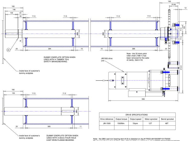
Note - the Ø65 cast iron bearing item # (9) is detailed on drg # FRSD/JM1500/BP/10179/005. The bearing fixings item # (10a), 10b), (10c) & (10d) are detailed on drg # FRSD/JM1500/BP/10179/005. The key for the safety brake option item # (11) is detailed on drg # FRSD/JM1500/BP/10179/005.
