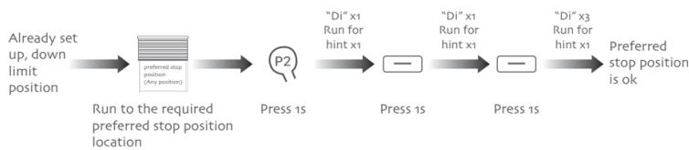
Note: Continuous moving mode, long press stop button, the curtain run directly from the current position to preferred stop position (Apply to the shade); Jog-move mode, long press stop button, the motor will first run to the down limit position, then run to preferred stop position (Apply to venetian blinds); Repeat this operation to remove preferred stop position.
